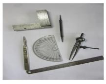
For hobby courses marking out is not too important, but to develop your skills you need to have marking tools such as a steel rule, scribe set square and protractor for working out angles. It is really important to use good quality dividers for marking arcs and circles. I also value a scalpel for marking straight lines.
