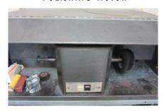
You can spend a fortune on a motor & extractor combination. But you can get by with a standard 2800 RPM I/5 HP motor (a slight variation is fine) Just make sure iyou can fit tapered spindles to fit the mops to. Also be aware that a lot of dust is generated, so mask up. My compound of choice is Hyfin for cutting and Rouge for finishing.
