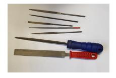
You can start your collection of files with a flat file and a half round ring file. There are different cutting grades, so start with a number 2 cut then add '0' cut files later.
