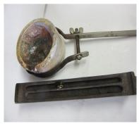
This is not essential for training but once you have a crucible and ingot mold you can salvage your scrap metal and reduce the need to keep buying stock gauge precious metals. This set up is only applicable if you have an oxy/gas set up.
