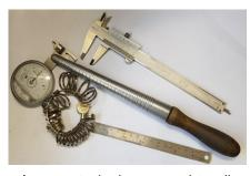
Accuracy is the key to good jewellery making. Traditionally jewellers would generally use a steel Vernier or caliper gauge but there are other options such as leverage gauge or spring gauge. Consider getting the digital or dial type vernier for easy use. They are not that expensive, your local hardware may have them. You will also need a ring size stick and finger gauge if you are making rings,
