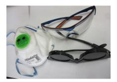
The most important thing in your workshop is your health and safety. Make sure you have the necessary safety gear on hand. Wear safely goggles at all times, wear a dust mask when using your drill, and extraction or ventilation should be in use over soldering and pickle areas.
