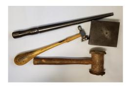
I recommend a steel ring mandrel and a chasing hammer for shaping and sizing rings, and for general forging I use a panel beaters hammer and clamp a flat stake into my bench vice. An anvil is good to have if you can find one.
