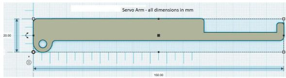
Hole diameter - 5 mm, thickness - 3 mm
