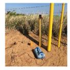
The <u>EM Signal transmitter</u> applies alternating current to underground cables and pipes which creates a detectable signal field. The transmitter is applied by means of direct connection or signal inductive broadcasting. The signal current constantly
