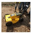
Ground penetrating radar, commonly called a GPR, is a noninvasive near surface geological investigation tool. In the locating industry, we use it to find buried pipes, cables, vaults, tanks, barrels and other buried objects.
